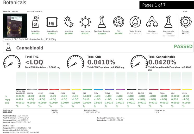
Cannabinoid analysis utilizing Ultra High Performance Liquid Chromatography with UV Detection (UHPLC-UV): Method SOP 300.23 for sample preparation and SOP 300.18b for analysis. Total THC = d8-THC + d9-THC + 0.877 \* THCA, Total CBD = CBD + 0.877 \* CBDA
